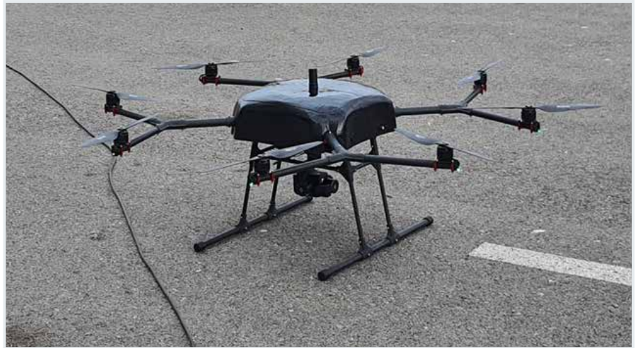
UAV assisted vehicle scanning based on thermal and high-resolution cameras
